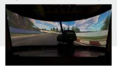
of a button. Regardless of the season, test scenarios for a wide range of conditions, including road surface, tire material and weather, can be run repeatedly, saving resources, wear and tear on the vehicle, and the need for a pit crew.
