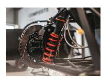
road or track use. This is also convenient when encountering speed bumps or steep driveways, enabling the vehicle's ride height to easily be adjusted by 15-60mm at the press of a button.
