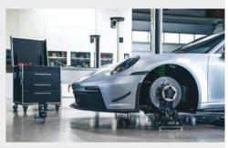
Drawing on its many years of experience in international motorsport, Manthey Racing has designed a wheel alignment system for motorsport vehicles and road cars, facilitating measurements locally or at events - even on uneven surfaces. Laser-based alignment pads guarantee precise leveling. All essential components, including the wheel load scale and the laser system, are enclosed in a portable flight case. See it for yourself at Manthey's booth at PMW Expo.
